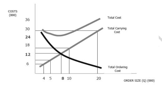
In the above graph line of total carrying cost intersects line of total ordering cost at 8,000 order quantities, where both of the costs are Rs. 12,000. At this order quantity the total cost is Rs. 24,000 which is the minimum most.
